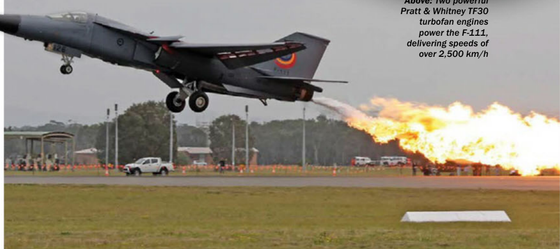
A Royal Australian Air Force F-111C performing a 'dump and burn' at an air show. The fuel is intentionally ignited using the aircraft's afterburner
